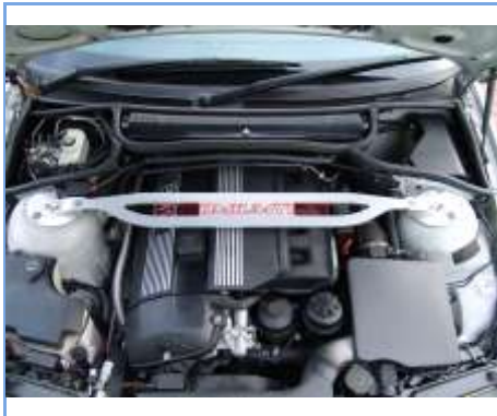
BMW E46 3-Series Aluminium Front Strut Brace Bar 6-Cylinder
